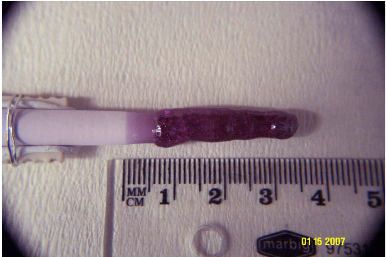
Figure 1: A ruby rod grown using the floating zone furnace.
